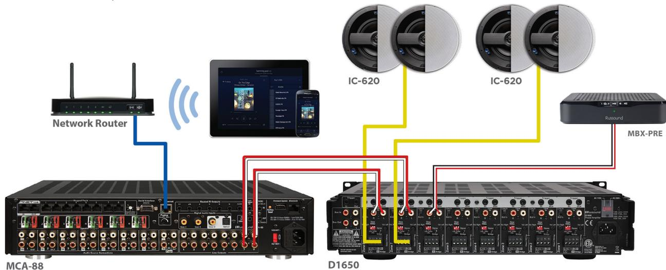
Using Bus input to share a source with multiple zones
