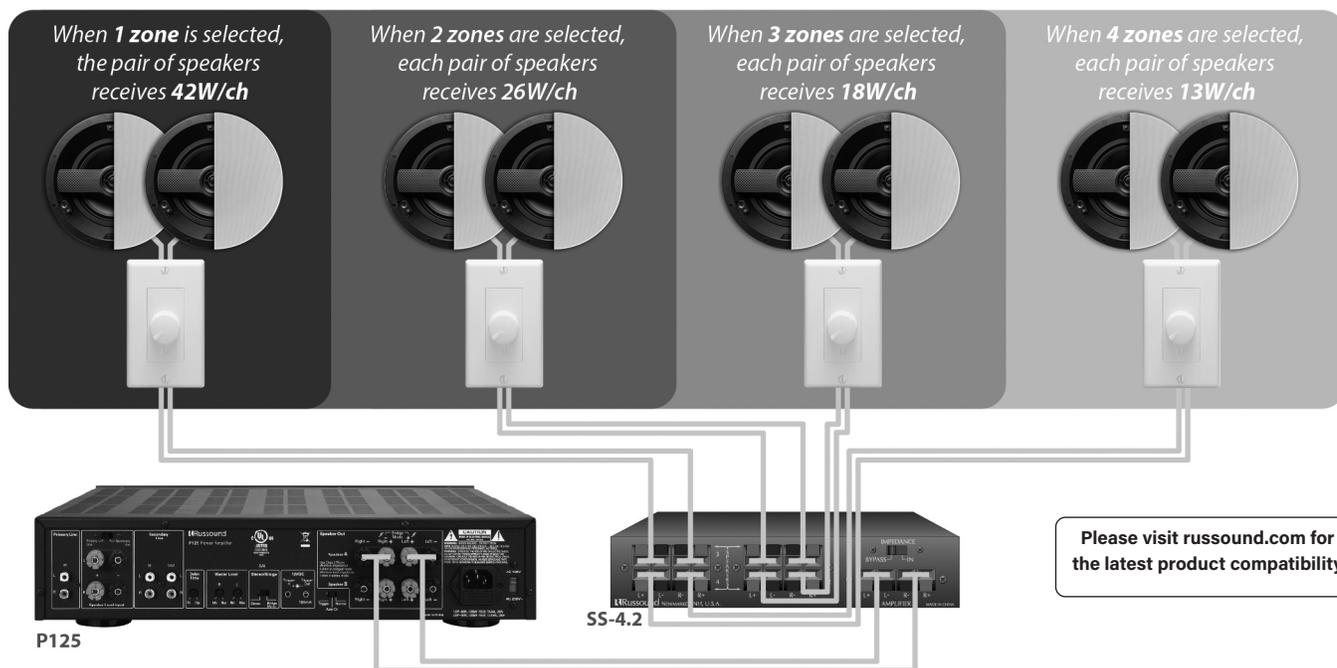
ALT-126R Volume Controls with impedance matching at 4X setting without speaker selector
