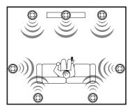
Make sure the speaker cutout is placed between two joists with plenty of clearance. Use a stud finder to locate joists, and mark locations. Be sure to avoid electrical wires and plumbing when cutting hole for installation. If you encounter electrical wiring or plumbing, you may have to consider another location.
