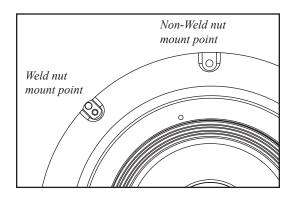
2.) Using 4 pcs - #10 x .05 in (12mm) sheet metal screw, attaching the baffle / driver to the back can. Be sure to match the mouting holes <u>without</u> weld nuts to clip nuts on back can.
