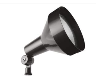
Large size flood for easier relamping and glare reduction. Durable one piece die casting with rugged mounting arm, weatherproof gasket and drain holes. Accepts 150 Watt PAR 38 max. Lamp not supplied.
