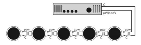
The total number of speakers multiplied by the tap value cannot exceed the output power (in watts) of the 70V/100V amplifier. The example below shows 5 total speakers. Using the 10W taps, you will need an amplifier with at least 50W (5 speakers x 10W tap). A good rule of thumb is to select an amplifier with 20% greater power; in this case, an amplifier that delivers about 62W.
