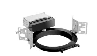
Easy to install 6" rough-in with die-cast aperture ring, removable driver, thermal protector and adjustable butterfly brackets. This rough-in is designed to make new construction recessed downlighting easy .
