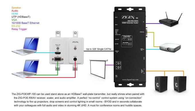
Example is showing our HDBaseT transmitter (ZIG-POEWP-100) connected to the HDBaseT receiver (ZIG-POE-RXAV) Amplified audio output for direct connection to speakers, LAN ports for almost anything you choose and for controlling/setting up the devices, relays, a 4K scaler and IR and RS232 control and functionality.
