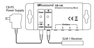
**Emitter Outputs:** Connect up to 4 emitters to the emitter jacks labeled 1-4 (green connectors).
